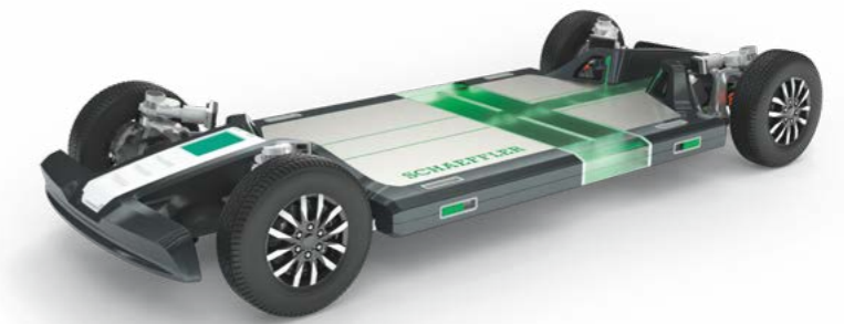
Rolling Chassis: One platform for all driving functions
