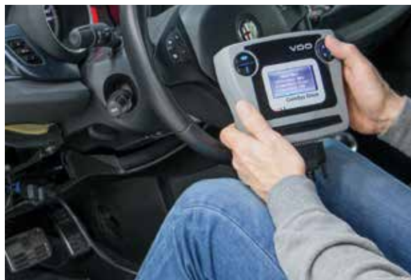
Basic adjustment with a suitable diagnostic tool
