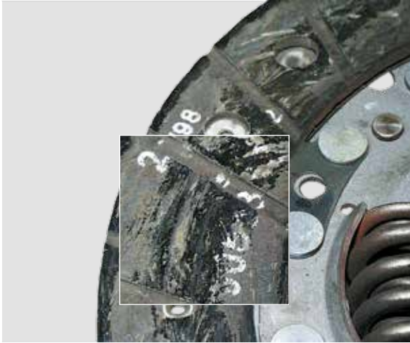
LINING SCORED ON THE FLYWHEEL SIDE
