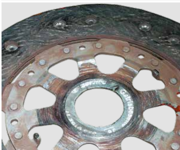
HUB OF THE CLUTCH DISK IS BROKEN
