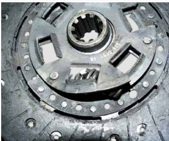
TORSIONAL DAMPER IS BROKEN
