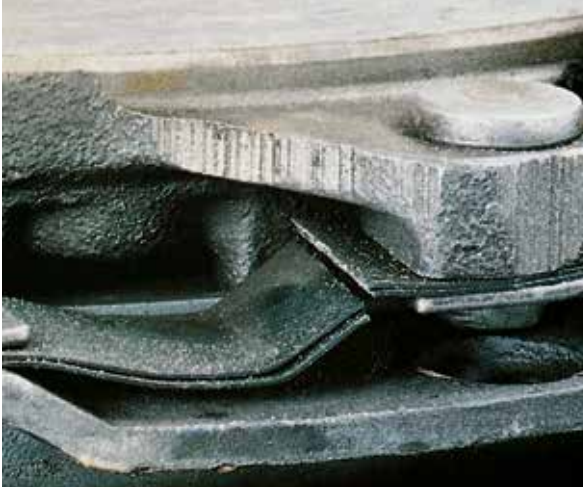
TANGENTIAL LEAF SPRING IS BROKEN
