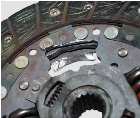
SPRING WINDOW IS WORN
