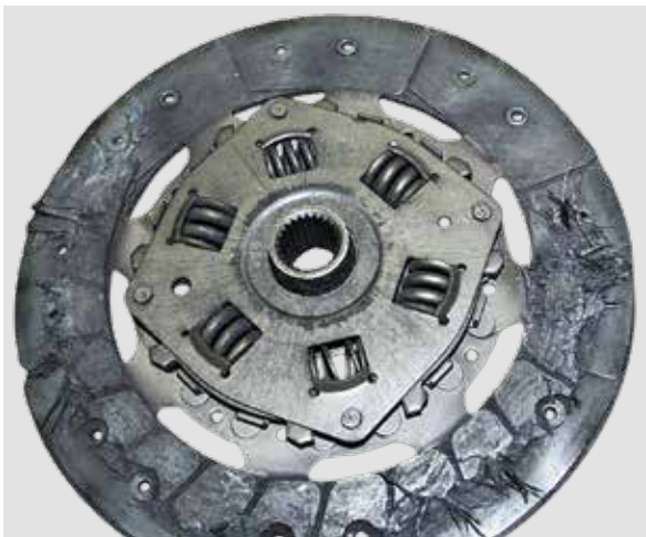
LINING IS BURNT OR HAS WORKED LOOSE
