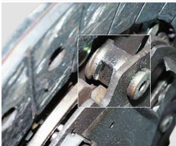
STOP PIN IN THE TORSIONAL DAMPER IS WORN
