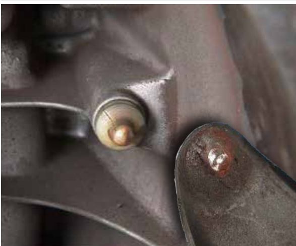
RELEASE FORK AND/OR BALL PIN IS WORN
