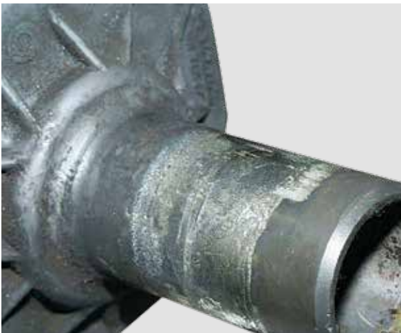
GUIDING SLEEVE IS WORN
