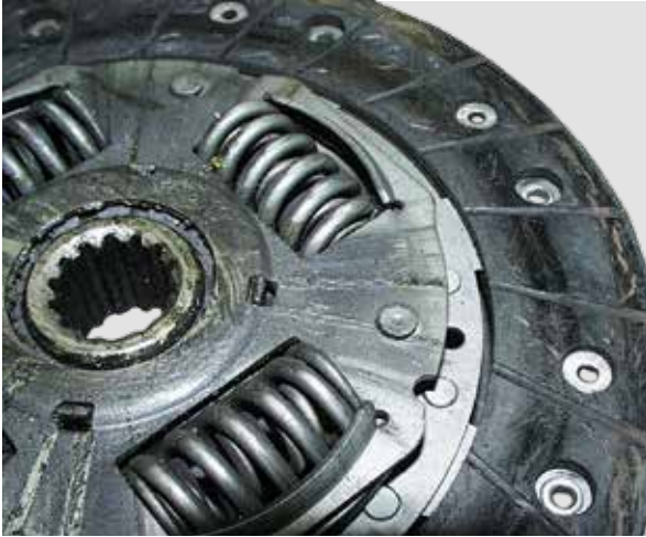
CLUTCH LINING IS OILY
