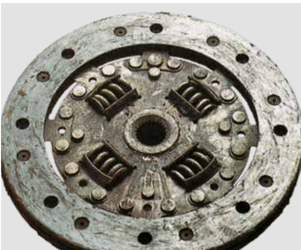
CLUTCH LINING IS OILY
