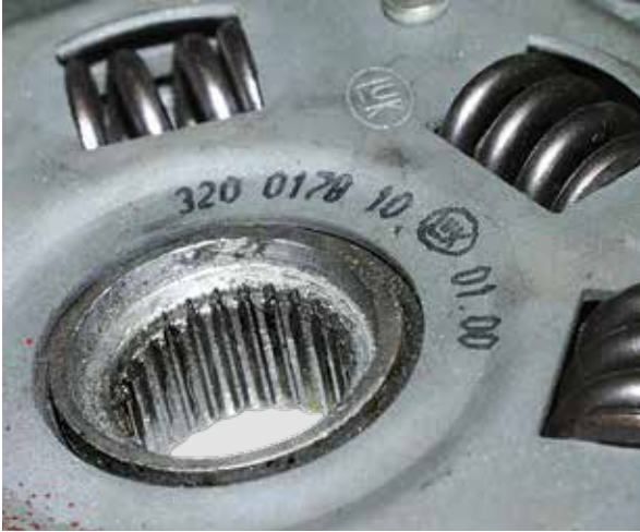
FRETTING CORROSION (RUST FILM) ON THE HUB PROFILE
