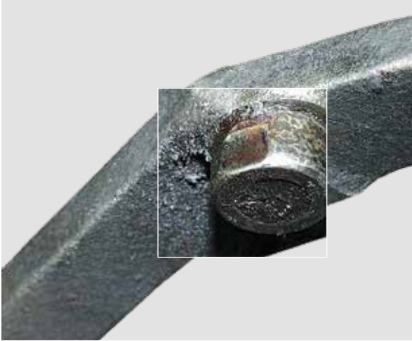
RELEASE BEARING SEATING ON THE RELEASE FORK HAS BEEN RUN IN
