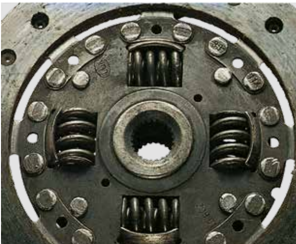
CONTACT TRACKS ON THE RIVET HEADS OF THE SEGMENT RIVETING (VW)
