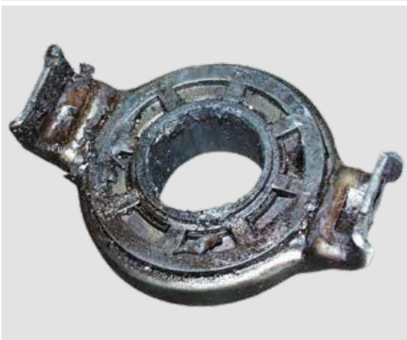
RELEASE BEARING SEATING IS WORN
