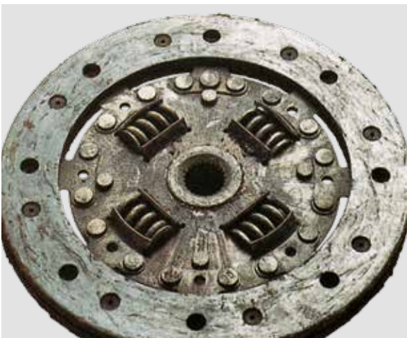
CLUTCH LININGS ARE COVERED IN EXCESS GREASE
