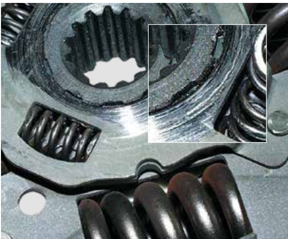
CONTACT TRACKS ON THE FIRST STAGE DAMPER
