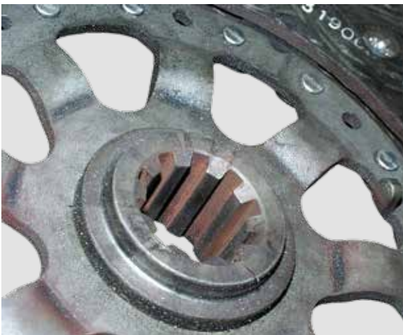
FRETTING CORROSION (RUST FILM) ON THE HUB PROFILE
