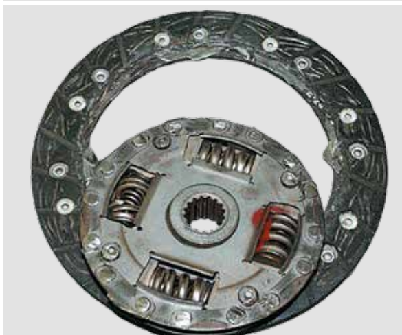
DISC ASSEMBLY IS BROKEN
