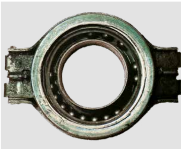
CONTACT BUSHING AND BALL BEARING ARE DESTROYED
