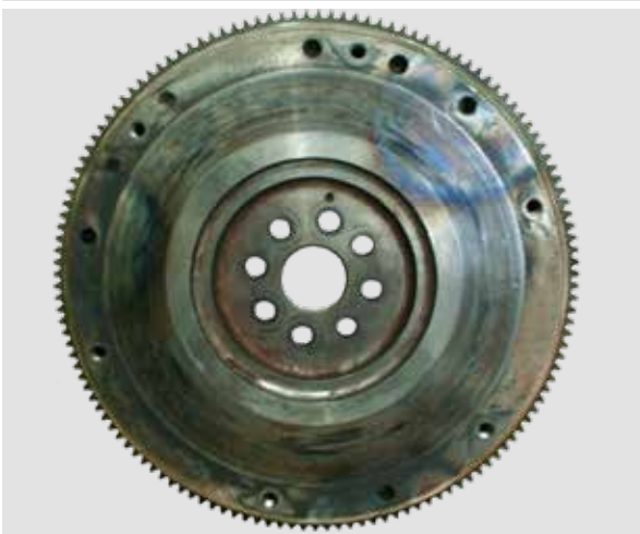
FRICTION SURFACE ON THE FLYWHEEL IS WORN
