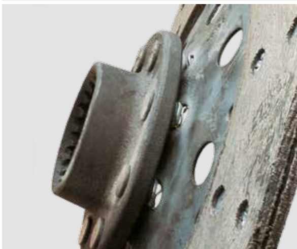
CLUTCH DISK HAS BECOME SAUCER-SHAPED
