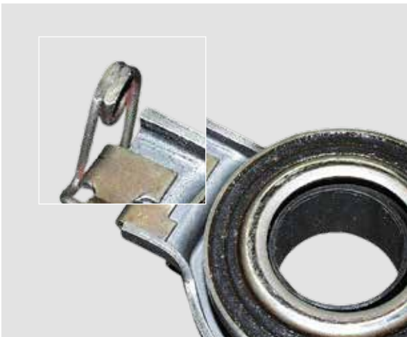
CONTACT TRACKS ON THE FORMED SPRING
