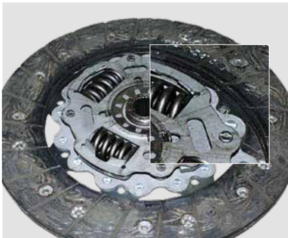
FRICTION LINING ON THE INNER RING IS OILY/ GREASY
