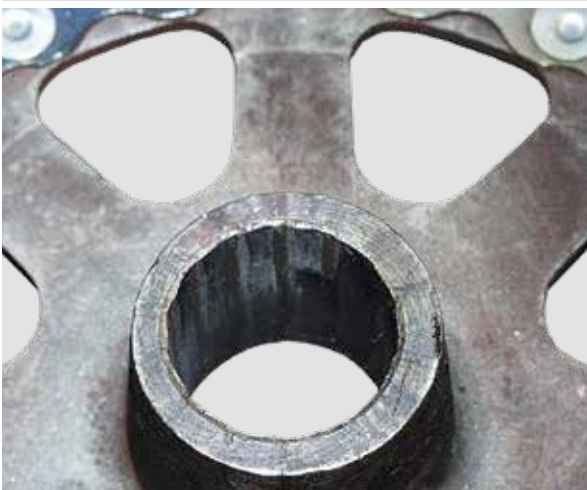
HUB PROFILE IS COMPLETELY MISSING
