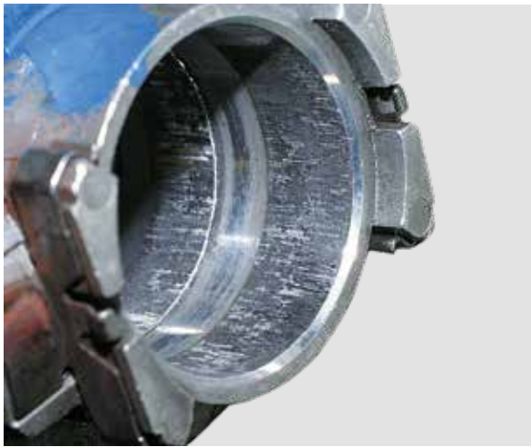
FRICTION LINING ON THE INNER RING IS OILY/ GREASY
