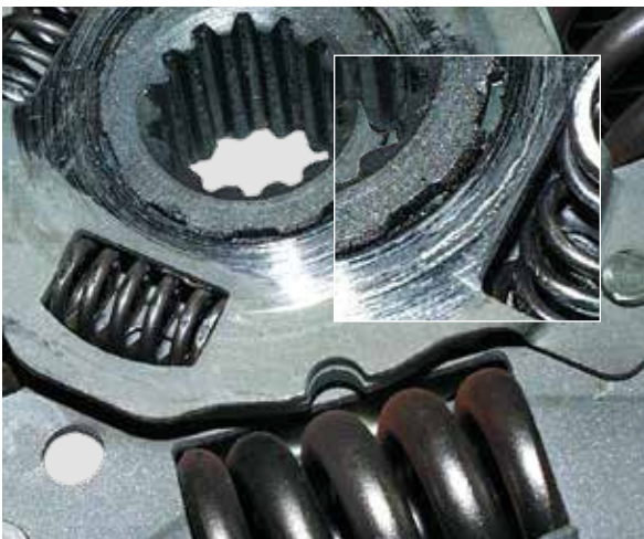
CONTACT TRACKS ON THE HUB OF THE CLUTCH DISK
