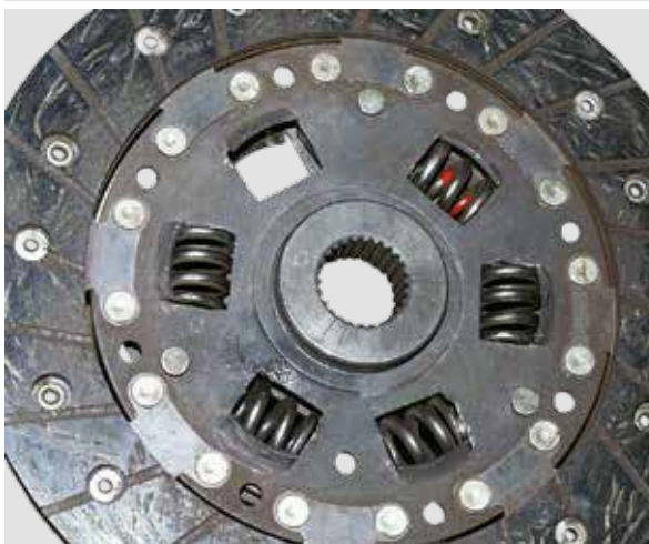
TORSION SPRING IS BROKEN
