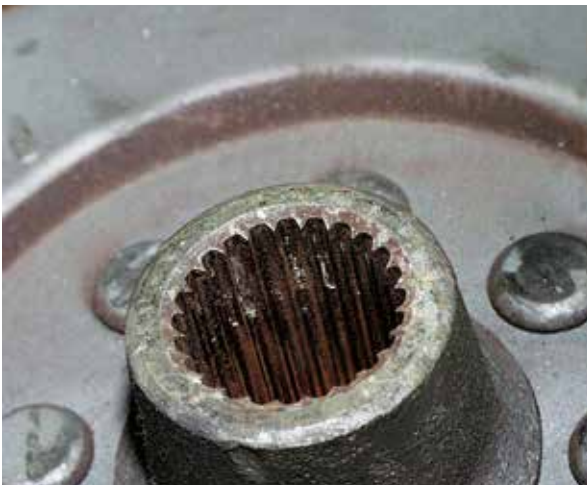
HUB PROFILE IS DEFORMED, TAPERED GEARING PROFILE
