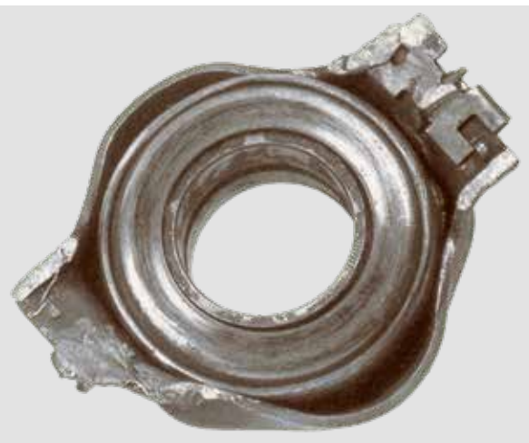
HOUSING OF THE RELEASE BEARING IS DEFORMED
