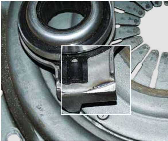
CONTACT TRACKS ON THE CLUTCH COVER AND RELEASE BEARING
