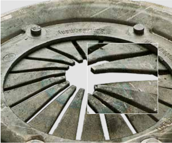
DISK SPRING TIPS ARE BENT
