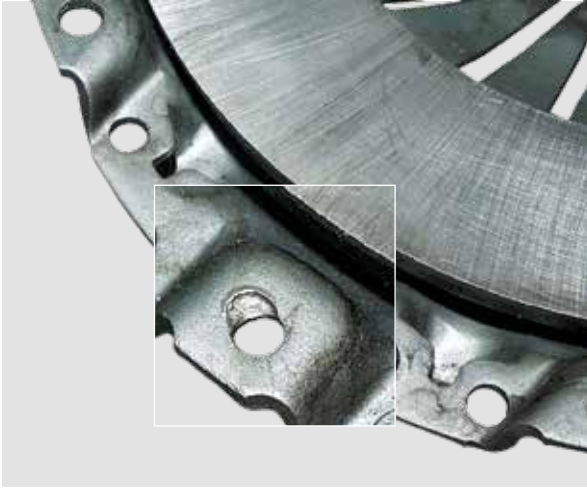
CLUTCH COVER IS DEFORMED
