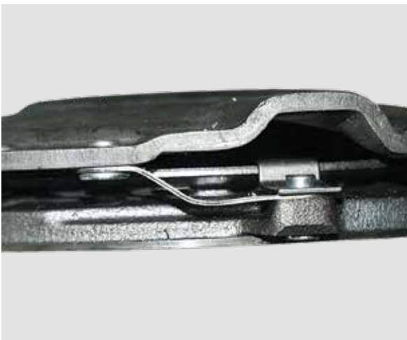
TANGENTIAL LEAF SPRING IS BENT
