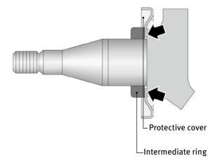
7. Position the wheel hub on the steering knuckle.
